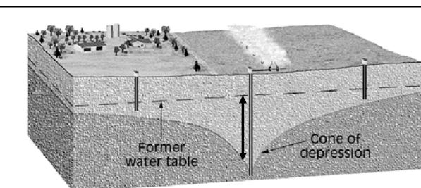
$$\text{水位降下量} = (\text{静水位}) - (\text{動水位})$$
