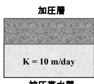
$$\begin{aligned} T &= K \times b \\ &= 10 \text{ m/d} \times 10 \text{ m} \\ &= 100 \text{ m}^2/\text{day} \end{aligned}$$
