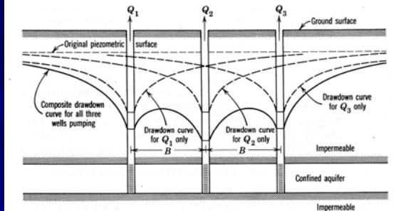
Fig. 4.27 Individual and composite drawdown curves for three wells in a line.
