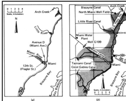
Fig. 14.19 Maps showing extent of seawater intrusion in and near Miami, Florida as of (a) 1904, and (b) 1959. Note the extent of intrusion associated with the drainage canals (after Kohout<sup>22</sup>; reprinted from the *Journal American Water Works Association*, Vol. 53, by permission of the Association, copyright © 1961 by American Water Works Association, 6666 West Quincy Avenue, Denver, CO 80235).
