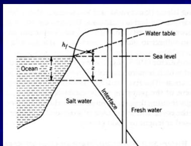
Figure 6.24 Hydrostatic conditions of the Ghyben-Herzberg relation.
